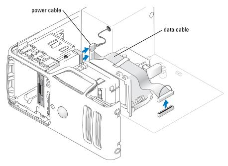
**3** Disconnect the power and data cables from the back of the floppy drive.
